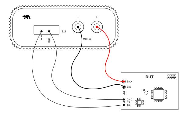
Set up Otii hardware, Otii Arc Pro, or Otii Ace Pro to capture logs from the DUT serial log.
