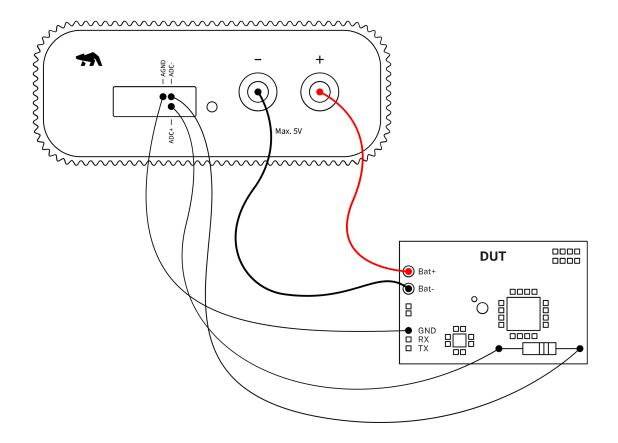
Set up **Otii hardware**, **Otii Arc Pro**, or **Otii Ace Pro** to measure a subsystem current and voltage over a shunt resistor in addition to measuring the complete system. Note that the resistor can be part of the actual system or applied externally.
