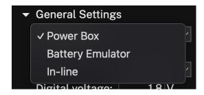
• Power Box: The Otii hardware will supply a constant voltage to the Device Under Test (DUT)
