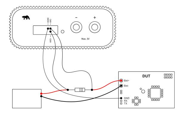
If the Device Under Test (DUT) needs to be powered from an external source while still measuring system current and voltage, an external shunt resistor connected to the ADC inputs of the **Otii** hardware, whether the **Otii** Arc Pro or **Otii** Ace Pro, can manage this.
