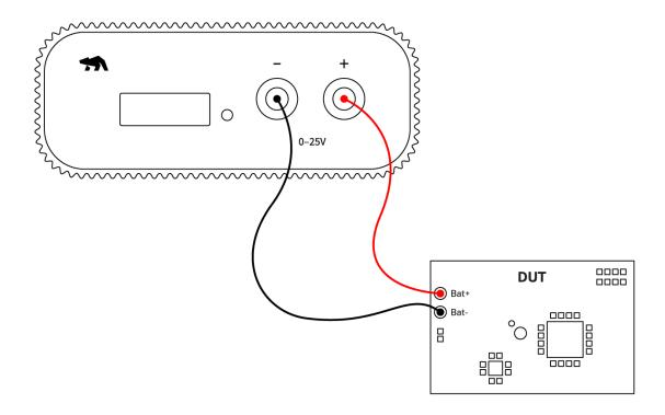
Set up **Otii hardware**, either the **Otii Arc Pro** or **Otii Ace Pro**, to work as a power source box providing constant voltage to the DUT, ranging from  $0.5\ V - 5\ V/0\ V - 25\ V$ , and enable it to measure output current and voltage.
